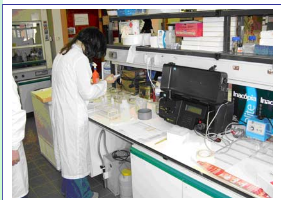
Photo 1. Fluorescence determination with use of spectrofluorometer.
